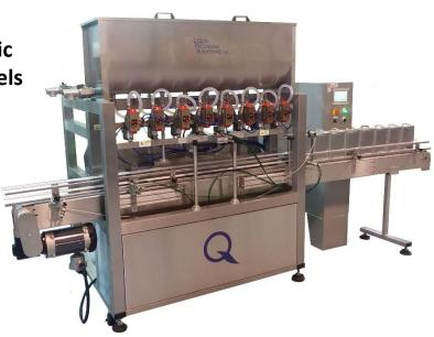
Pump Filling Machines are time or pulse based filling systems that use individually controlled pumps to move product. One pump on each fill head allow the machines to handle a range of product viscosities. Pump fillers may be used to fill foods, personal care products, lubricants, gels, oils, products with particulates and more!
